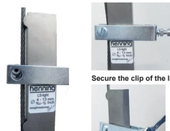
Secure the clip of the load sensor
